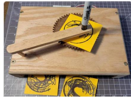
**Simple Turntable Drawing Machine With Arduino**
