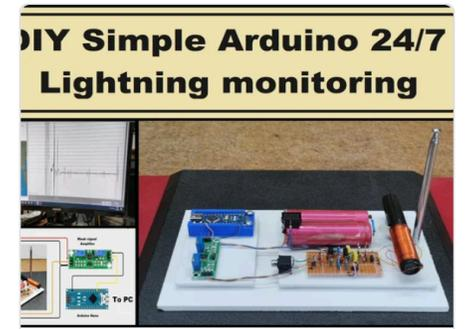
**DIY Simple Arduino 24/7 Lightning Monitoring System With Graph and Data Logging**
